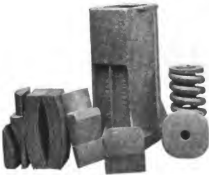
Fig. 3960. Gould Friction Draft Gear, Dismantled.
